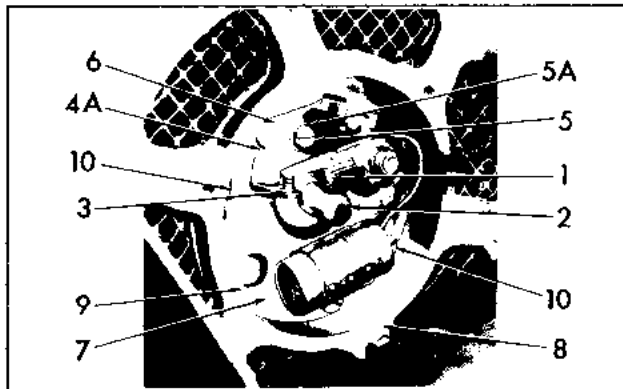
Figure 5F-11B. Circuit Breaker, 1971 & Later Models
